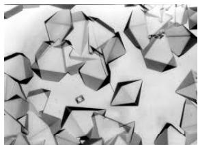
For synchrotron single crystal diffraction experiments crystals are typically 10 – 100 microns in size ( $1\mu\text{m} = 1 \times 10^{-6}\text{m} = 10,000\text{\AA}$ )
