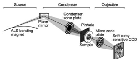
**Figure 1** | A diagram of the soft X-ray microscope XM-1. The microscope uses a micro zone plate to project a full field image onto a CCD camera that is sensitive to soft X-rays. Partially coherent, hollow-cone illumination of the sample is provided by a condenser zone plate. A central stop and a pinhole provide monochromatization.
