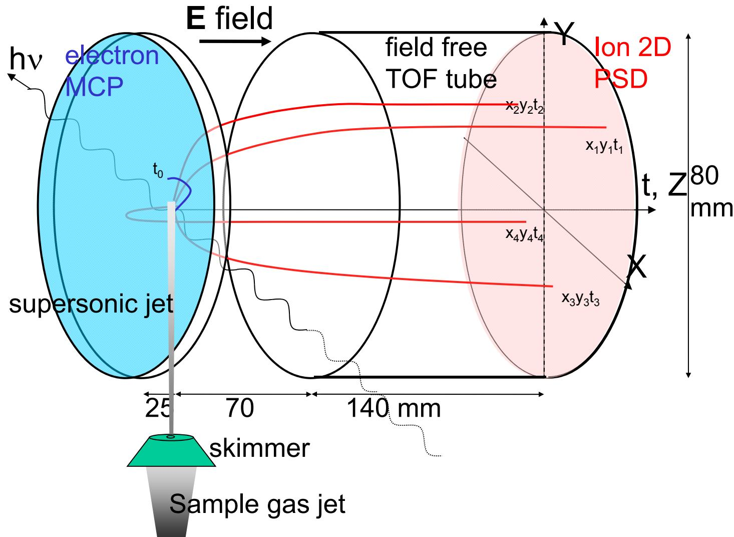
position & time of flight ( $x,y,t$ ) → 3D momentum of each particle
