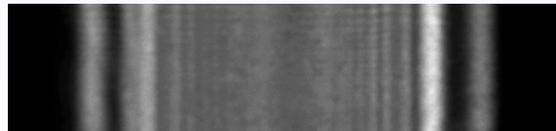
Reflection image of SACLA XFEL from double mirrors with small particles
