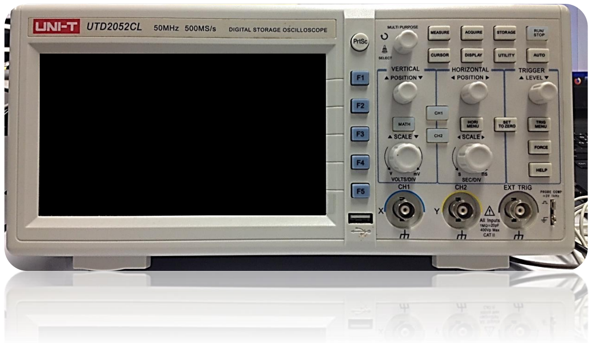
UNI-T UTD2052CL Dual-Channel Digital Storage Oscilloscope (50MHz)
