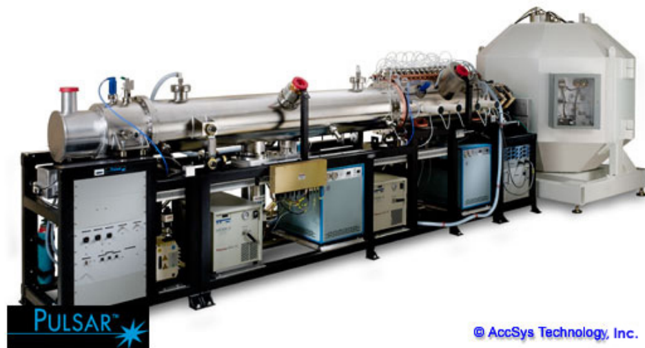
Figure 11: The AccSys PULSAR compact proton linac system [17]. The modular assembly shows the ion source and RFQ on the left, followed by the Alvarez DTL, and culminating in the locally shielded target station on the right.
