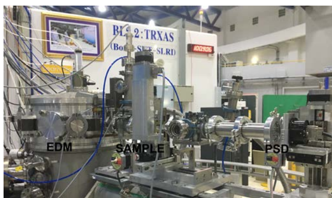
Figure 2: Photo of the TRXAS end-station showing, from left to right, an EDM, a three-axis stage, and a 1024 channels NMOS linear image sensor.
