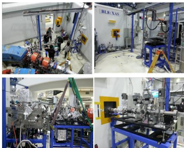
Figure 2: Removal of front-end and downstream components of Beamline 8 (upper panels); installation of a new front-end beam diagnostic chamber, collimating mirror chamber, and a downstream beam diagnostic chamber (lower panels).
