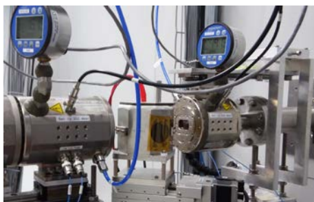
Figure 9: The octagon furnace available at the BL1.1W. The furnace has been developed for XAS experiments both in transmission and fluorescence modes and is capable of raising the temperature up to 750 °C.
