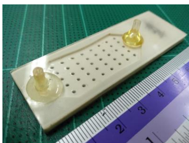
Electrostatic micro-well by non-toxic polymer clay
