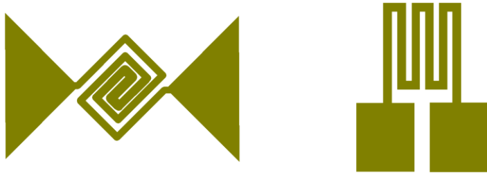
Design of \mu -hotplate (temperature sensor)
